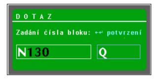
By means of the push-button s with numbers the required block No. is to be entered. The block No. may consists of maximum eight digits. when entering further numbers, the higher digit places disappear. By this method it is possible to correct the eventually erroneously entered block No. so that it is added by the zeroes until the window will be empty.
