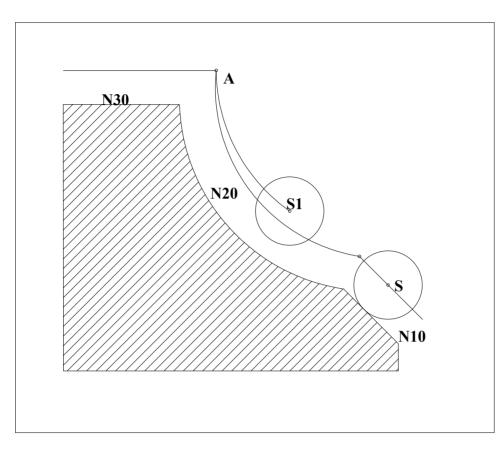
On the above figure, the tool path with the radius "r" is illustrated. When selecting the N20 block from any
