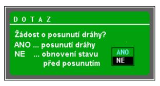
down of the "displacement" push-button (see the figure), because the system has to know, if required the displacement by further value or the displacement has to be cancelled. comfirming with When YES the displacement by one value will be performed. When confirming NO. al displacement will be lost and the program will be returned back to the programmed path on the end of the next block. If
